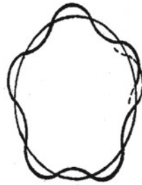
Fig. 18.—Motion of a wave in a circle; a single definite wave form is only possible when the circumference of the circle is a whole number of times the wave-length.
